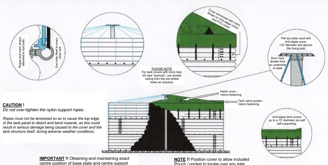
centre position of base plate and centre support pole is critical to ensure correct fitting and securing of the tank cover.
