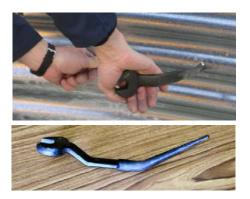
19mm socket for parabolts
