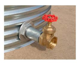
Screwed Outlet Assemblies These are available in 2", 3" and 4" and screwed Male BSP, providing a thread to take a filter assembly on the inside of the tank and a screwed gatevalve on the outside of the tank. The panels are provided with predrilled holes to customer specification and the outlet assemblies are installed so that the liner and tank panels are trapped between backing flanges.
